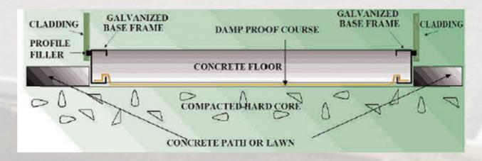
This section below shows a typical building without a base frame. Damp will seep in from the sides as the concrete is exposed to the outside elements.
